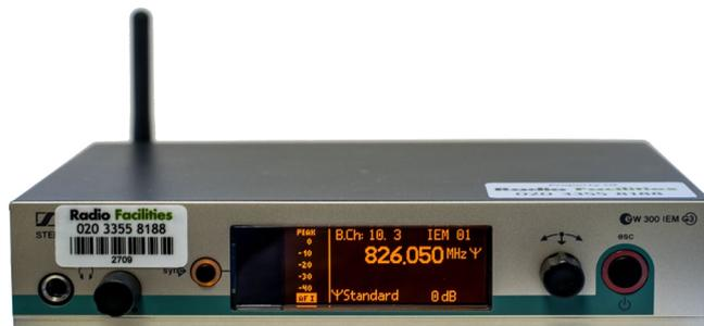
Sennheiser IEM mains-powered transmitter
